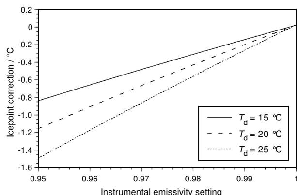
**Figure 8.** Expected reading for an 8–14  $\mu\text{m}$  IR thermometer as a function of instrumental emissivity setting when viewing an ice-point blackbody cavity with effective emissivity of  $\epsilon_{bb} = 0.999$ . The ambient temperature is  $T_{amb} = 20$   $^{\circ}\text{C}$ .
