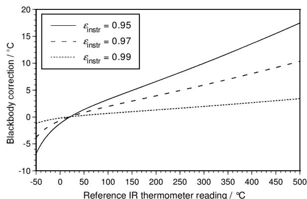
**Figure 7.** Corrections required to the readings of a reference IR thermometer aimed at a blackbody calibration source when calibrating an 8–14 μm IR thermometer with a detector temperature of  $T_d = 20$  °C and with instrumental emissivity as given on the graph. The reference thermometer also operates from 8–14 μm and its instrumental emissivity is set to 1.
