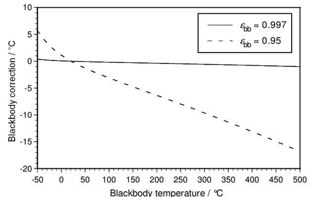
**Figure 5.** The solid line is for the same conditions as Figure 4, except that the emissivity setting on the IR thermometer is  $\epsilon_{instr} = 1$ . The dashed line is for a flat-plate calibrator with emissivity of  $\epsilon_{bb} = 0.95$ , again for  $\epsilon_{instr} = 1$ . For both curves, the blackbody corrections are independent of the detector temperature.
