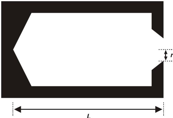
**Figure 2.** A blackbody cavity of length  $L$  and aperture radius  $r$ , whose walls have an emissivity  $\epsilon_s$ . The effective emissivity of the cavity is given by equation (10). In use, the cavity is heated uniformly in a furnace or dry-block calibrator.
