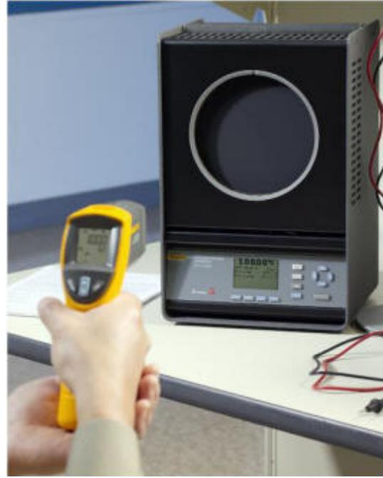
**Figure 3.** A flat-plate calibrator being viewed by an infrared thermometer. Photo courtesy of Fluke Corporation, Hart Scientific Division, reproduced with permission.
