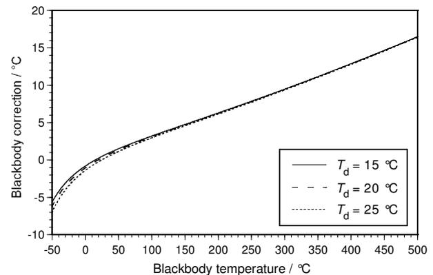
**Figure 4.** Corrections to the temperature of a blackbody calibration source, whose effective emissivity is  $\epsilon_{bb} = 0.997$ , to give the expected reading for an 8–14  $\mu\text{m}$  IR thermometer with a fixed emissivity of  $\epsilon_{instr} = 0.95$ . The ambient temperature is assumed to be  $T_{amb} = 20^{\circ}\text{C}$  and the detector temperature is as given on the graph.
