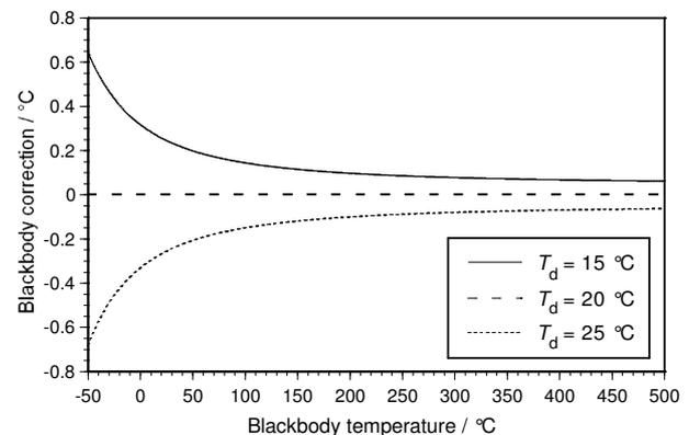
**Figure 6.** Same conditions as Figure 4, but for an IR thermometer with an emissivity setting of  $\epsilon_{instr} = 0.95$  viewing a flat-plate calibrator with emissivity of  $\epsilon_{bb} = 0.95$ . When  $T_d = T_{amb} = 20^{\circ}\text{C}$ , the blackbody corrections are zero for all temperatures.
