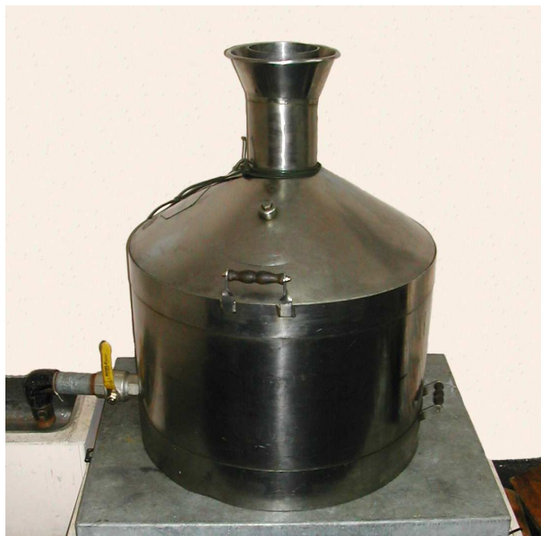
Figure 3. A 220 L reference standard volume. The vessel is on a 1 m wide platform scale.
