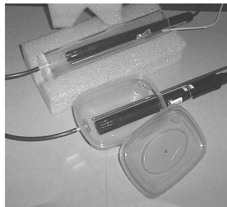
Figure 2. Examples of test chambers. Note thermometer probe and thermal insulation. Lid is removed from air-tight container for clarity.
