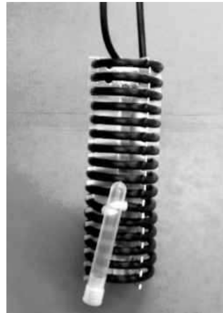
Figure 1. The saturator coil showing the water trap and inlet and outlet tubing.
