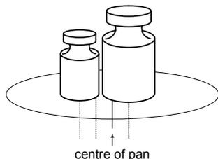
**Figure 8.** Centring two unequal weights. When used together, a 50 g weight is placed twice as far from the centre of the pan as a 100 g weight.
