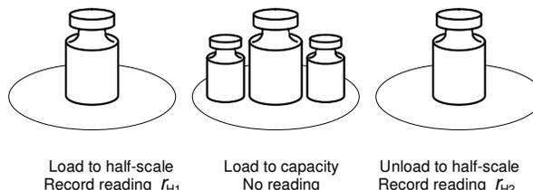
**Figure 5.** Illustration of a hysteresis measurement.
