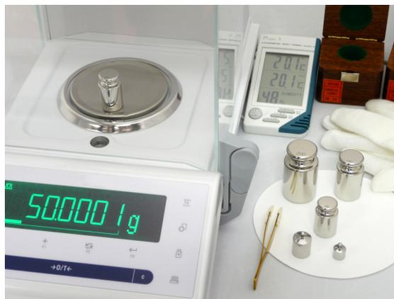
Figure 2. Setup for balance calibration, showing pan position error measurement.
